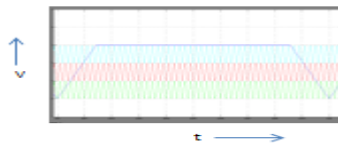
Figure 6: Shape of trapezoidal wave for 7 th order Harmonic Elimination
