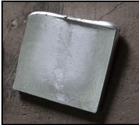
Figure 3: As Casted Specimen
