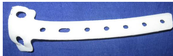
Figure 8: Custom implant for position 1 fabricated using FDM
