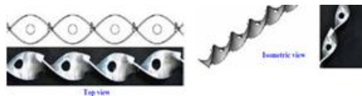
Figure 2: Perforated Twisted Tape with Parallel wings [3].
