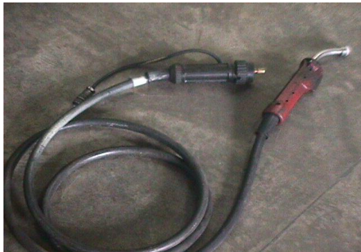
Figure 5: CO 2 welding torch
