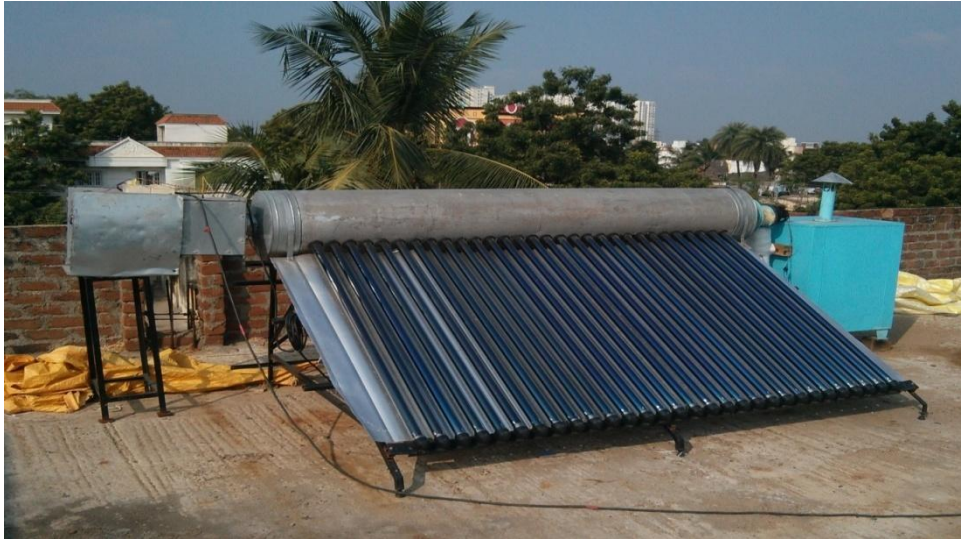
Figure 2: Experimental setup with Aluminium sheet Reflector
