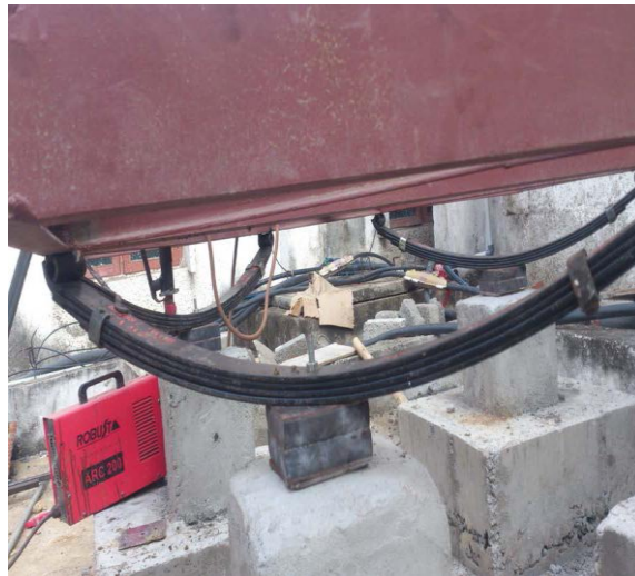
Figure 6: Assembly of column, bearing and leafspring
