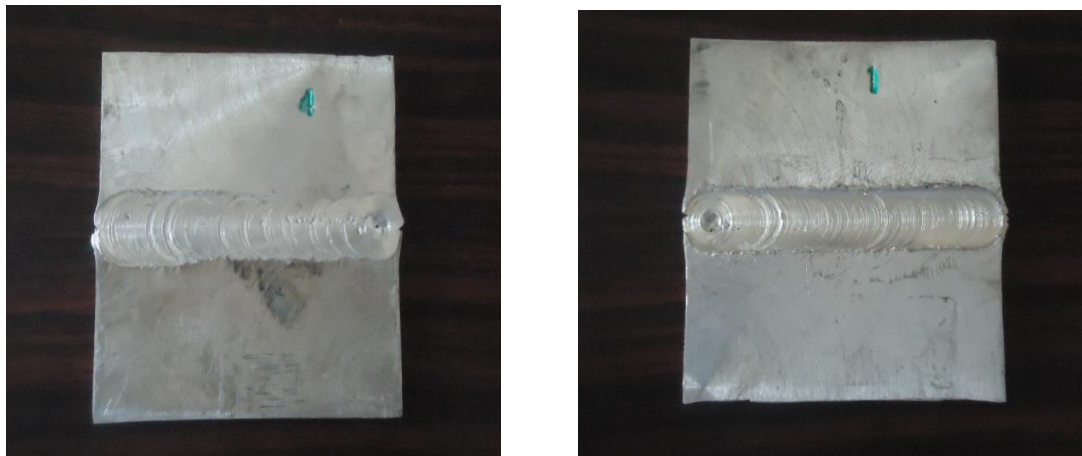
Figure 4: Photos of the top surfaces of as – welded specimens
