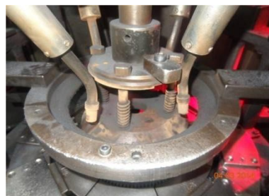
Fig.2 Welding fixture table
