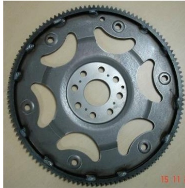
Fig.1 Ring gear / Flex Plate Assembly
