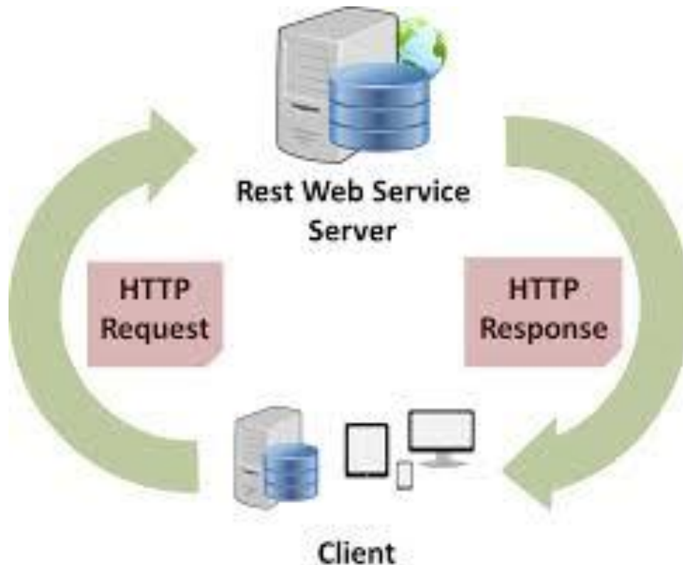
Figure 2 Rest Web Service flow diagram
