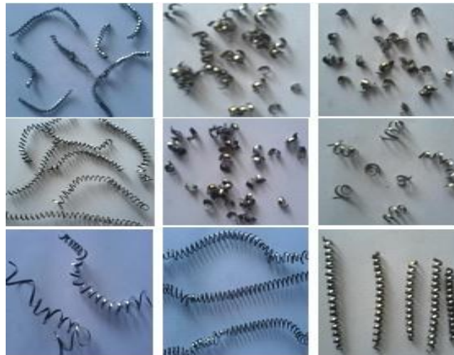
Fig 8 Chip Formation Mode In Dry Machining
