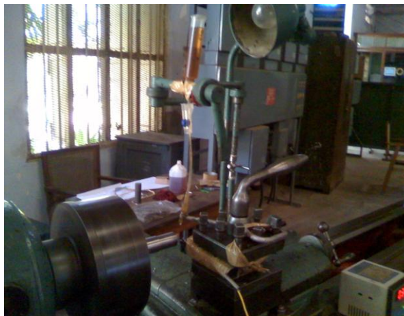
Fig 1 Minimum quantity lubrication setup
