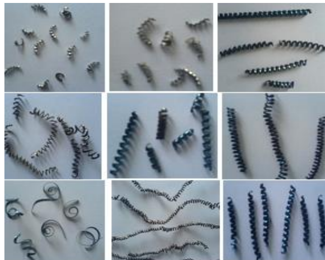
Fig 6 Chip Formation Mode In Wet Machining
