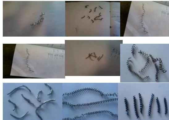
Fig 4 Different modes of chip formation in MQL
