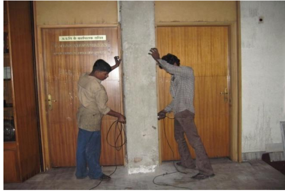
Fig. 3.3: Column testing by direct transmission
