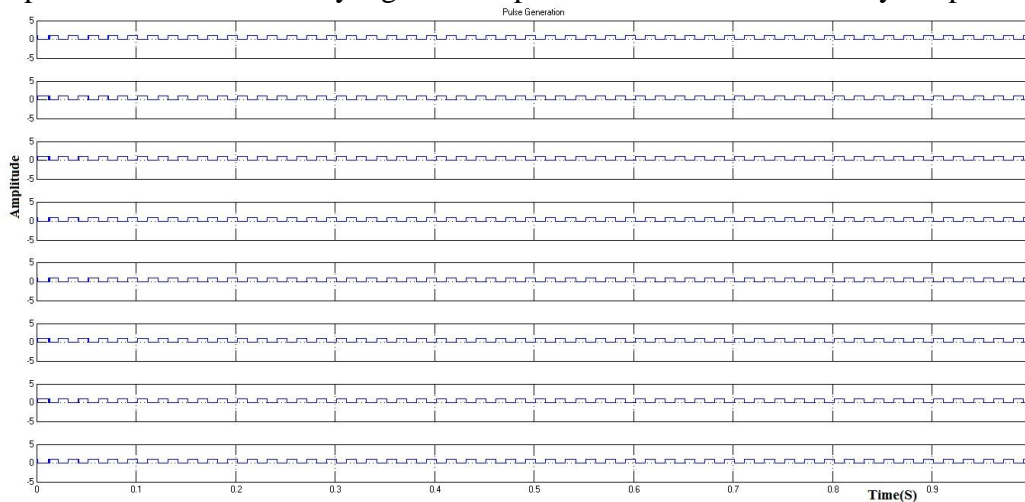
Fig.6. Gate Pulses for Seven Level Inverter
