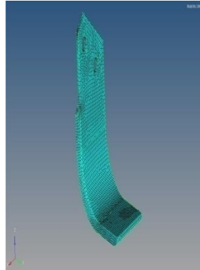
Fig .10 Meshed Existing blade
