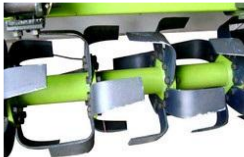
Fig.5 Rotavator blade fixed with flange
