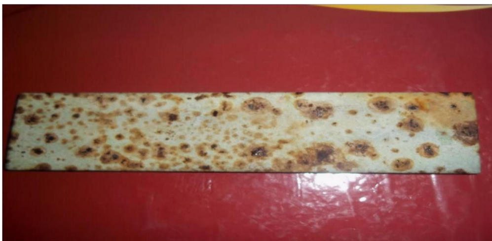
Figure 9: Uncoated sample in salt spray test
