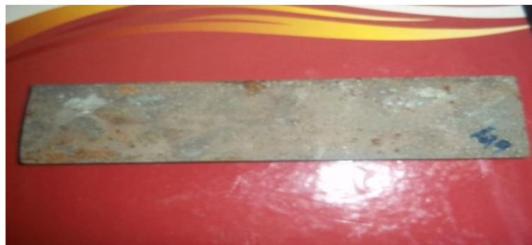
Figure 8: coated sample in salt spray test
