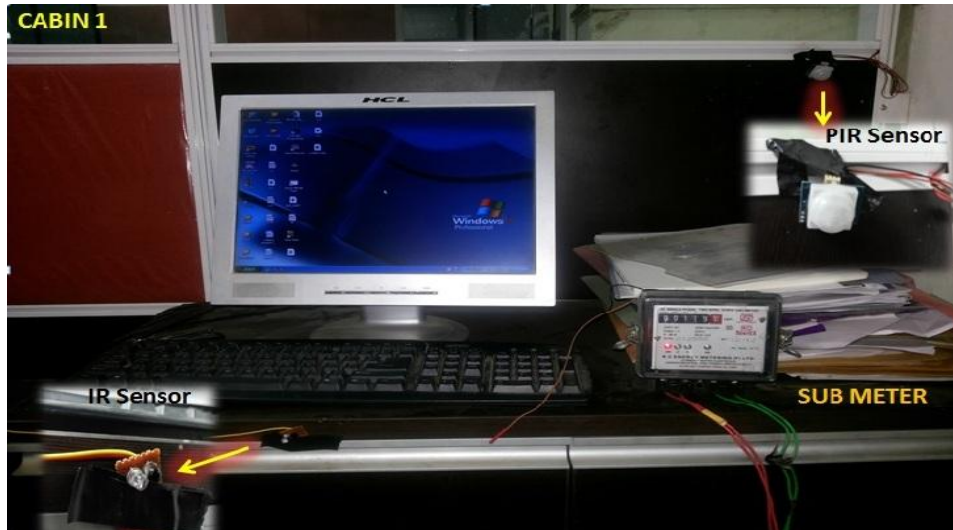
Fig.7. Deployment of PIR and IR in a Cabin
