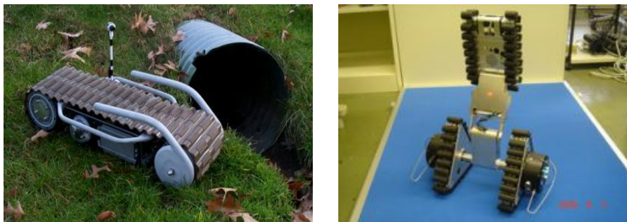
Fig. 8: (a)Aurora [34] of Hagen Schempf (b) SRN1 [35] of AIST using Track Belt Locomotion
