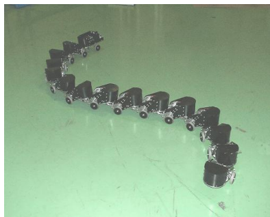
Fig.5: Articulated Cord Mechanism Serpentine Robot R3 developed by Shigeo Hirose[32]
