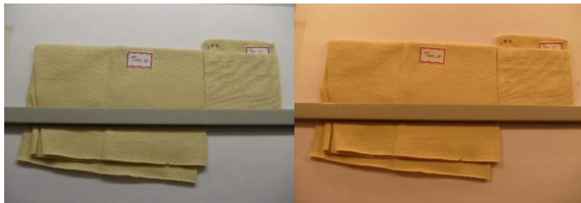
Figure 10: Photographs of Knitted Target and the Matching sample at different illuminants
