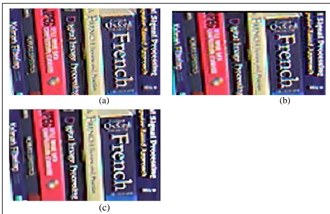
Fig:6. Reconstructed Images from the Book_case1_small tracked video using a) Single image SR reconstruction using sparse b) SVD based SR using blind deconvolution c) Reconstructed image using Proposed algorithm
