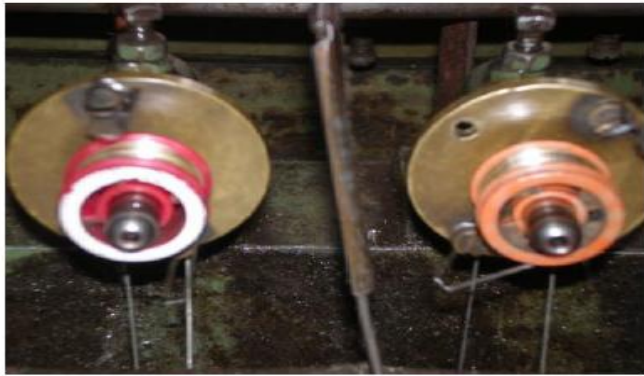
Perforation on the flywheel
