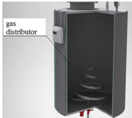
Fig. 1 The bio-reactor with barbotage pipeline in the form of spiral
