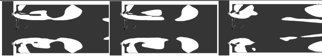
Fig.9. The scalar field of Q-criterion at different moments of time in the longitudinal section of the channel behind the diaphragm (dark color marks the areas with Q < 0 , white color marks the areas with Q > 0 )
