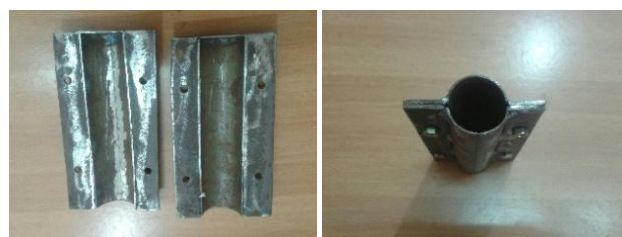
Fig.1. Mould for preparation of specimen
