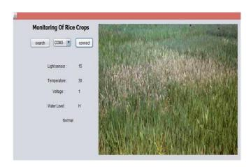
The above figure is the output observed on the laptop. For this initially we have to select the COM3 port and connect to the receiver kit through UART and USB connector. The video of the field is received and observed using TV tuner card.
