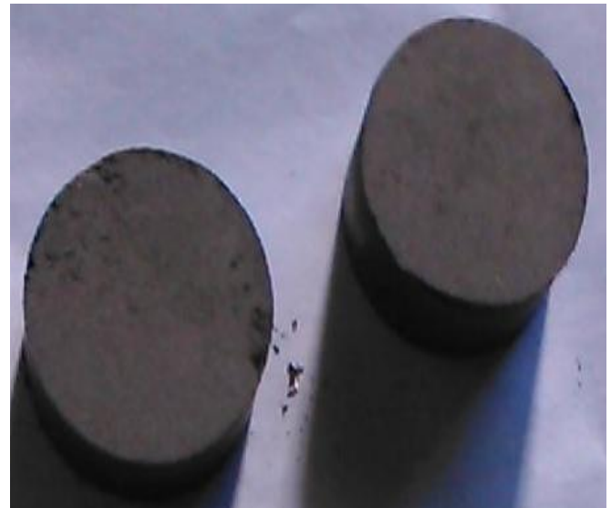
Fig.2.1 Specimen before sintering
