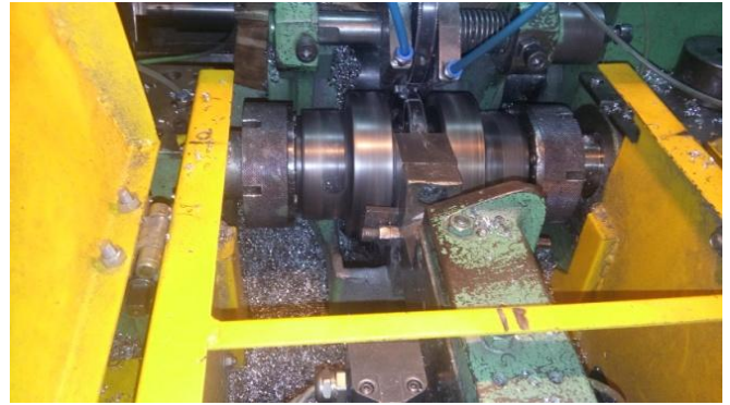
Fig.3. Machining of bimetal bearing
