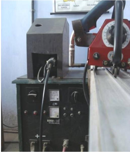
Fig. 2 Setup of GMAW unit
