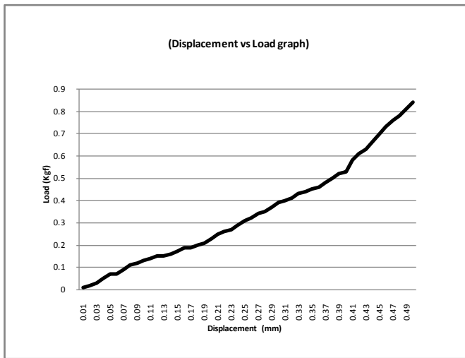
Fig.2 Bellow compression test
