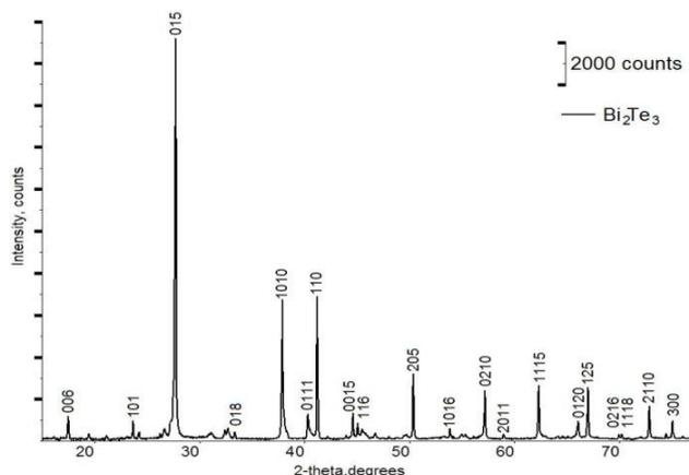
Figure 1. XRD pattern of the Bi<sub>2</sub>Te<sub>3</sub> powder.
