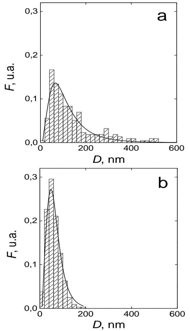
**Figure 5.** Histograms of the grain size distributions for the bulk  $\text{Bi}_2\text{Te}_3$  material sintered at the HPIP-temperature of 573 K and various  $P$  values: 2 (a) and 8 GPa (b). Solid lines are fits to the lognormal distribution.
