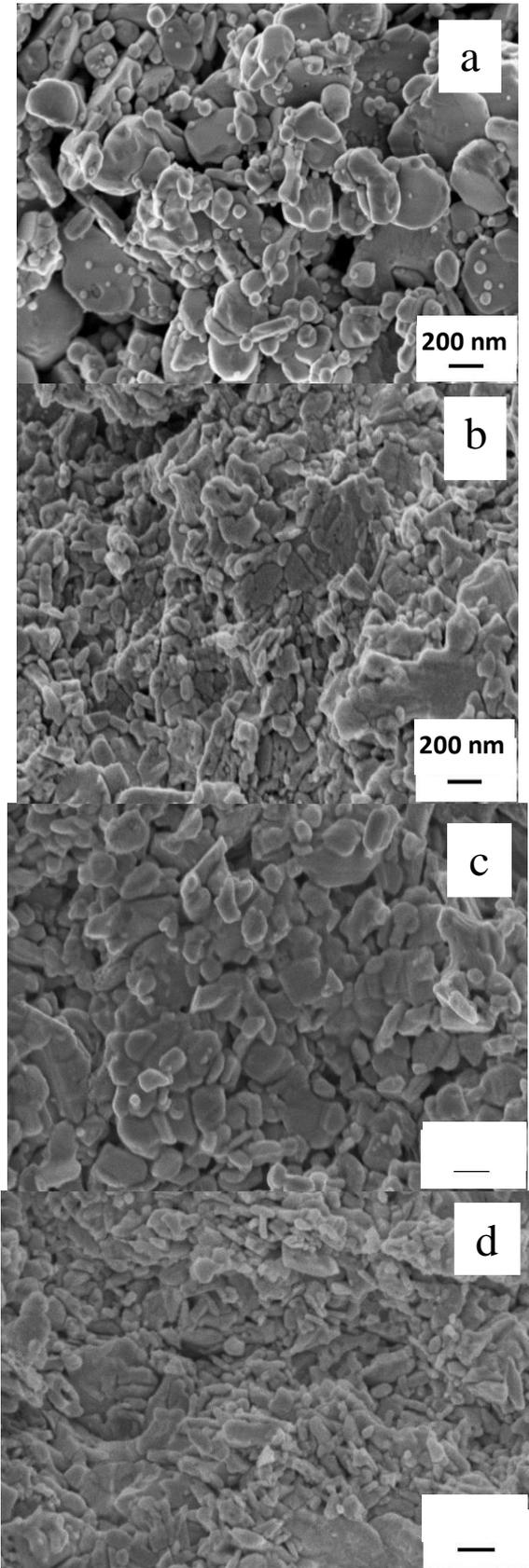
**Figure 4.** SEM images of the bulk  $\text{Bi}_2\text{Te}_3$  nanomaterial sintered at the HPIP-temperature of 573 K and various HPIP-pressures: (a) 2, (b) 4, (c) 6 and 8 GPa (d).
