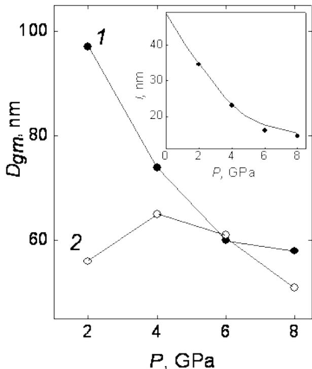
Figure 6. The  $D_{gm}(P)$  dependences for the HPIP-temperatures of 573 K (curve 1) and 673 K (2). The inset is the  $I(P)$  dependence.
