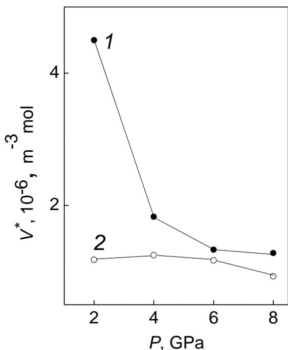
Figure 7. The  $V^*(P)$  dependences for the HPIP-temperatures of 573 K (curve 1) and 673 K (2).
