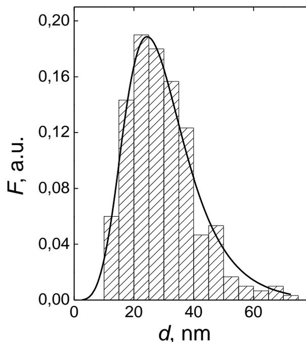
Figure 3. Histogram of the Bi<sub>2</sub>Te<sub>3</sub> nanoparticles size distribution.
