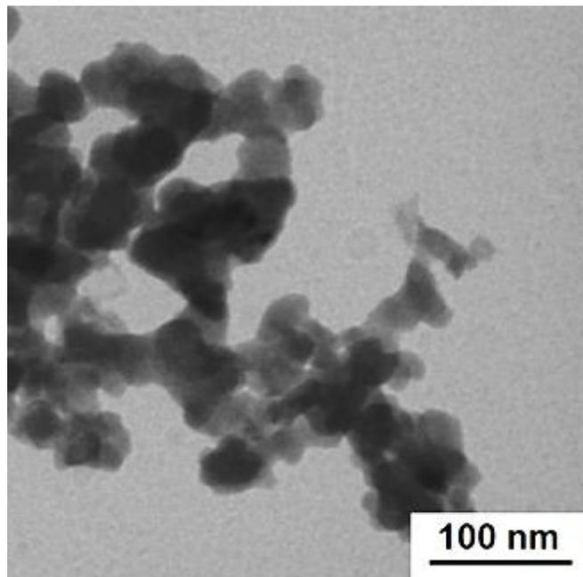
Figure 2. TEM image of the Bi<sub>2</sub>Te<sub>3</sub> nanopowder.
