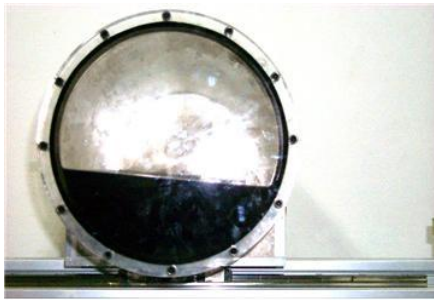
Fig.5. Determination of Natural Frequency of Sloshing Resulting from Horizontal Vibration in Lateral Direction
