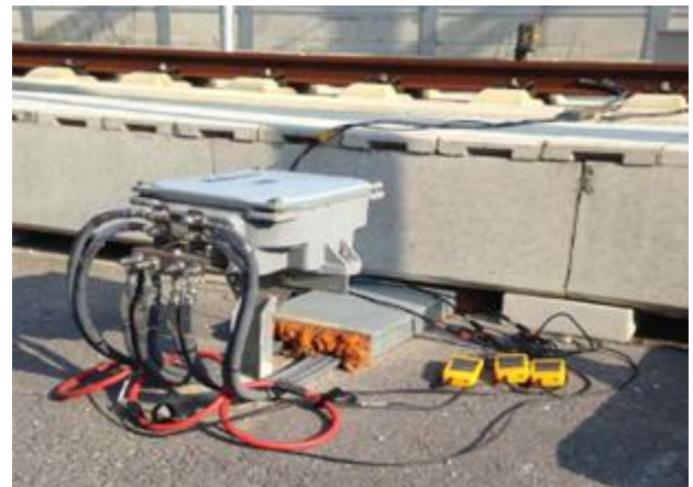
Fig.1. Installation of Rogowskii coil
