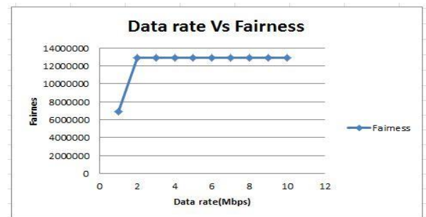
Fig. 20. Data rate vs. fairness between two links of TFRC
