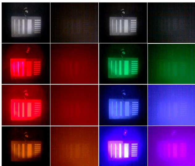
Figure 7 – Images of the test plate in the camera, with and without fog, illuminated with the light with different wavelengths taken by the Web-camera
