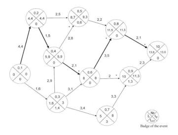
The Rice 1. Processed network graph oriented telecommunication network of the data exchange (the fat line is shown critical way of the issue to information)
