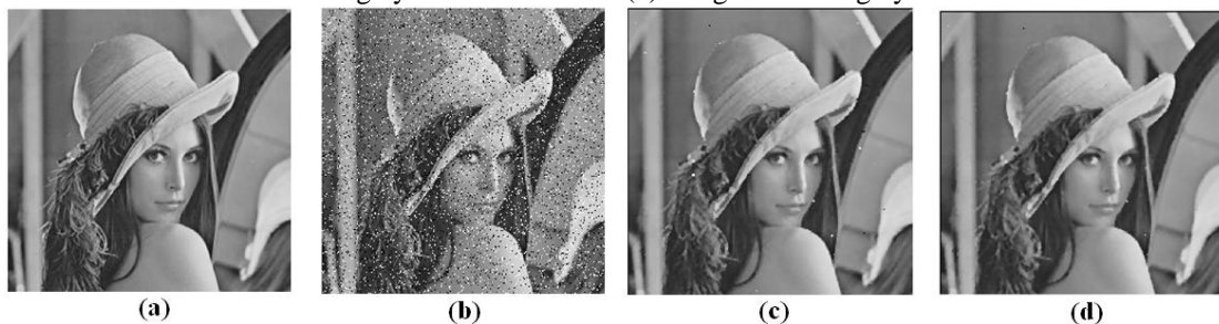
Fig. 3. Comparative of Image Quality using 3X3 Mask (a) The original Image (b) Degraded Image 10% Noise (c) Image Denoising by Standard Median (d) Image Denoising by CMF.
