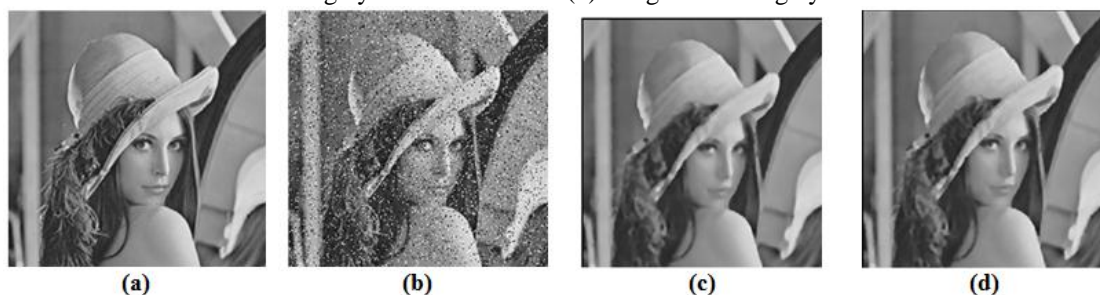
Fig. 4. Comparative of Image Quality using 5X5 Mask (a) The original Image (b) Degraded Image 10% Noise (c) Image Denoising by Standard Median (d) Image Denoising by CMF
