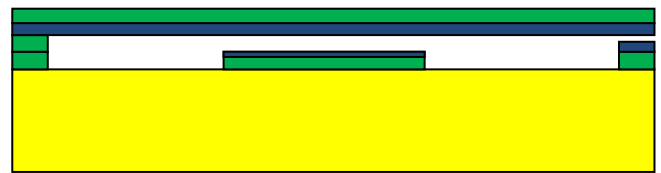
Fig.2. Cross section of typical MEMS cantilever switch [Liu 2007]
