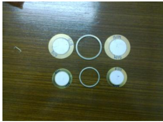
Fig. 2. The piezoelectric buzzer elements with steel rings
