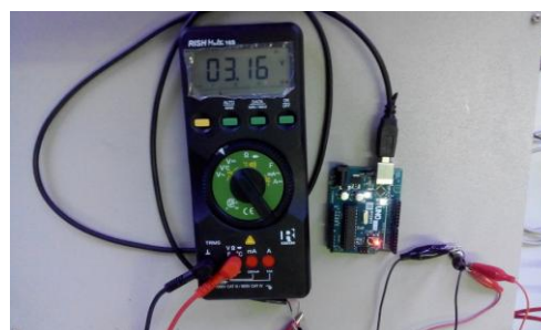
Fig. 9. Arduino board powered by the supercapacitor
