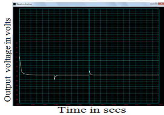
Figure.10 closed loop response of BFOA-PI Controller with sudden disturbances of \pm 20\% of rated load at 0.01sec and 0.02sec.
