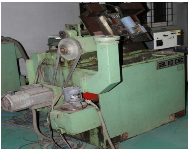
Figure 3.The SBL110 CNC machine retrofitted with open controller.
