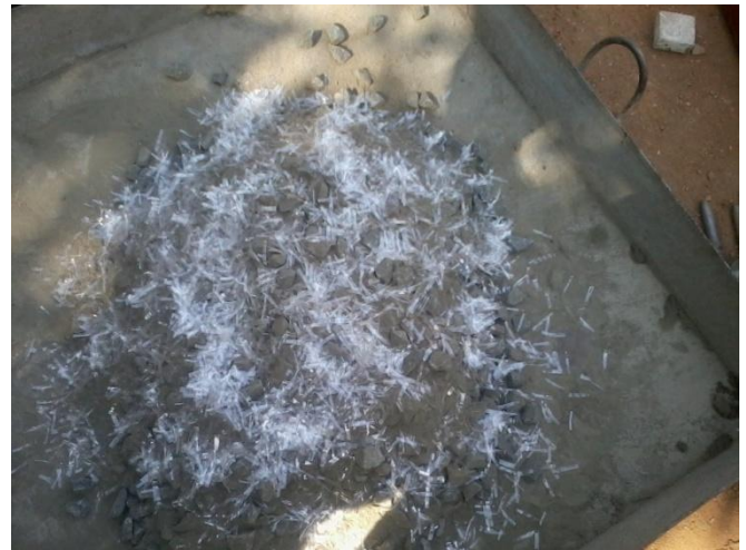
Fig. 2. Pet Fibre Addition in Concrete
