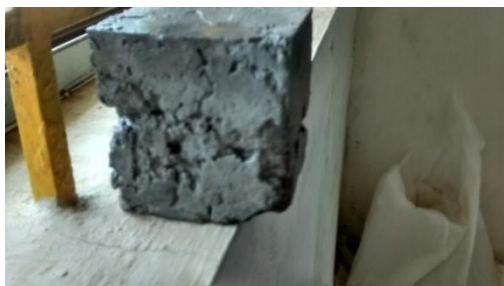
Fig-8 GPC specimen after 6 weeks of chloride attack
