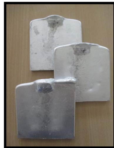
Fig 2. Cast plate of Al- TiB_2 - ZrB_2 MMC
