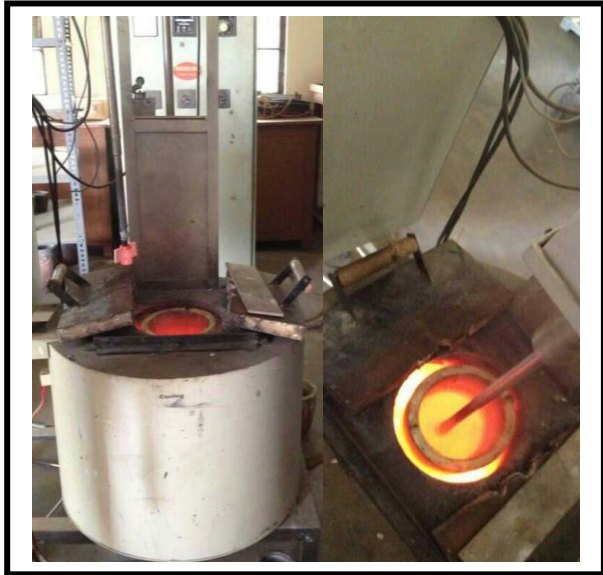
Fig 1. Typical Stir Casting Furnace showing the Stirrer in Operation.
