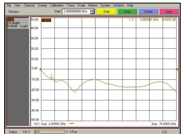
Fig.11. Measured Frequency response of the prototype with respect to (a) Return Loss (S11).
