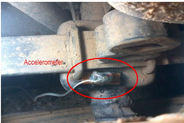
Figure 5 MEMS Accelerometer fixed on the axel
