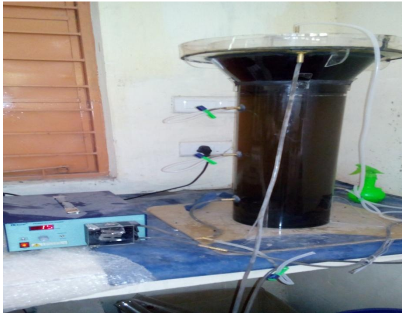
Figure 1: Up flow Anaerobic Sludge Blanket Reactor (UASBR) – A laboratory scale model
