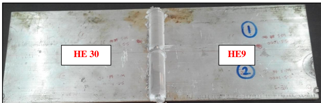
Figure 3: FSW of Aluminium alloy HE30 and HE9
