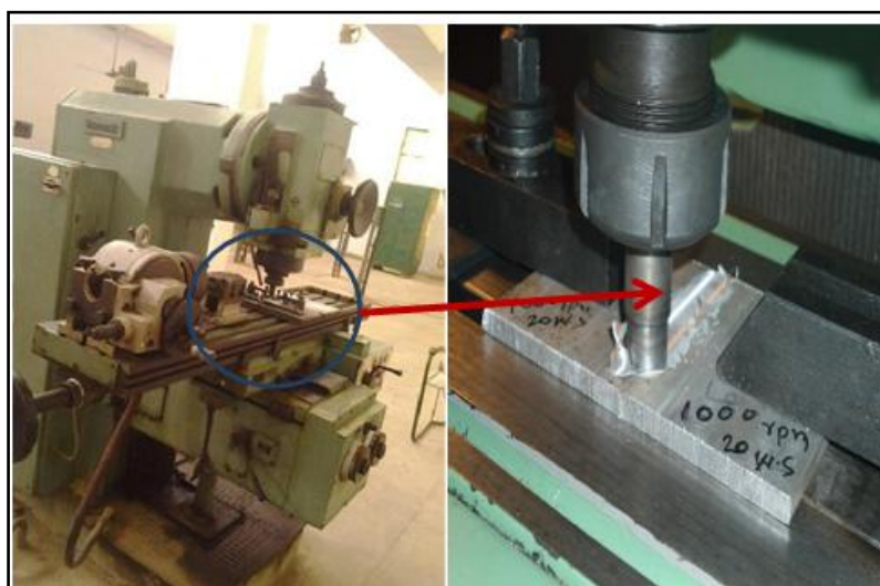
Figure 1: FSW Experimental Setup
