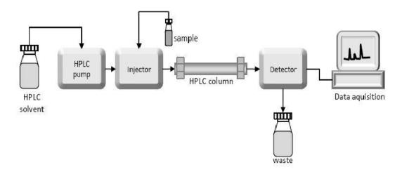
**Diagram 1** The layout of HPLC components. For up-scaling from analytical scale to preparative, the difference is the size of column diameter.
