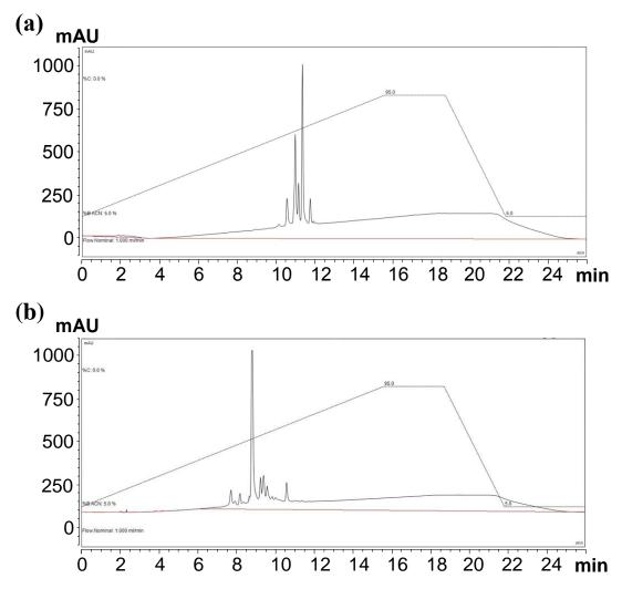
**Figure 2:** Chromatograms for a full range of polarity gradient (a) fraction no. 10; (b) fraction no. 23.
