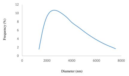
Figure 4. Particle Distribution of TiO<sub>2</sub> Nanoparticles
