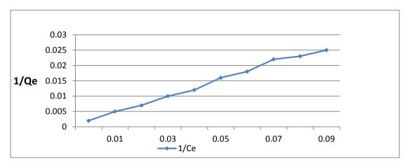
**Figure 5.** Langmuir adsorption isotherm of the adsorbents for Norfloxacin (Temperature =  $450 \pm 1$ , rotations per minute= $400\pm 1$ , adsorbent dose= 31.9mg, equilibrium time = 30 minutes pH=6)
