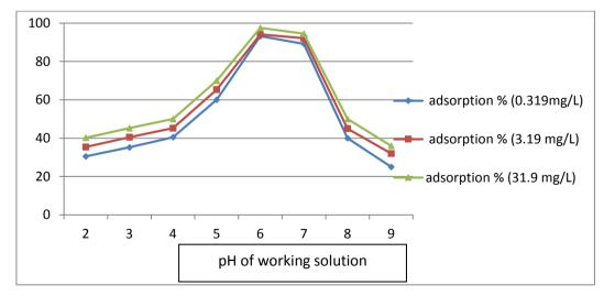
Figure 4. % Adsorption vs. pH in different concentration of adsorbate
