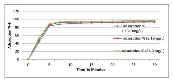
Figure 2 % Adsorption vs. contact time and different concentration of adsorbate
