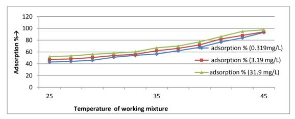
Figure 3. % Adsorption vs. temperature and different concentrations of adsorbate
