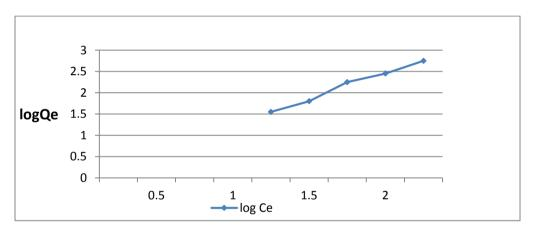
**Figure 6.** Freundlich adsorption isotherm of the adsorbents for Norfloxacin (Temperature =  $450 \pm 1$ , rotations per minute= $400\pm 1$ , adsorbent dose= 31.9mg, equilibrium time = 30 minutes pH =6
