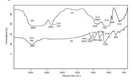
Figure 4. FTIR spectrum (a) cellulose from corn cobs [3] (b) PANI [11].
