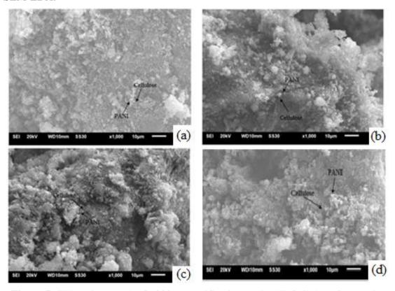
**Figure 7.** SEM micrograph of 1000x magnification (a) PANI-Cellulose Composite without Swelling and sonication (b) Swelling and Sonication methods(c) Swelling method (d) Sonication method
