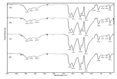
**Figure 5.** PANI-Cellulose composite FTIR spectrum (a) without swelling and sonication methods (b) swelling and sonication methods (c) swelling method (d) sonication method
